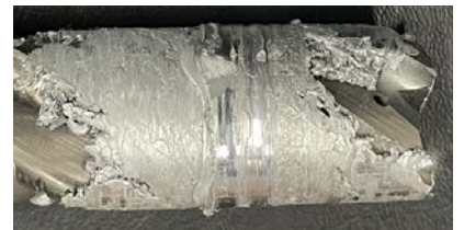
Old Endmill with Build Up
